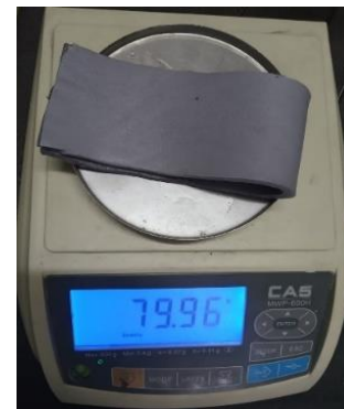
Fig. 5. Weigh the samples on a laboratory scale before and after compression
