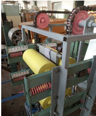
Fig. 1. Experimental stand of a vertical type roller machine that squeezes liquid from wet tannery semi-finished products
